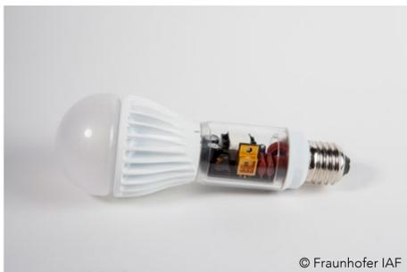
Figure 2: LED retrofit lamp as alternative to classical light bulbs. Left: LED retrofit lamp with an energy-efficient driver based on gallium nitride, developed at Fraunhofer IAF.
